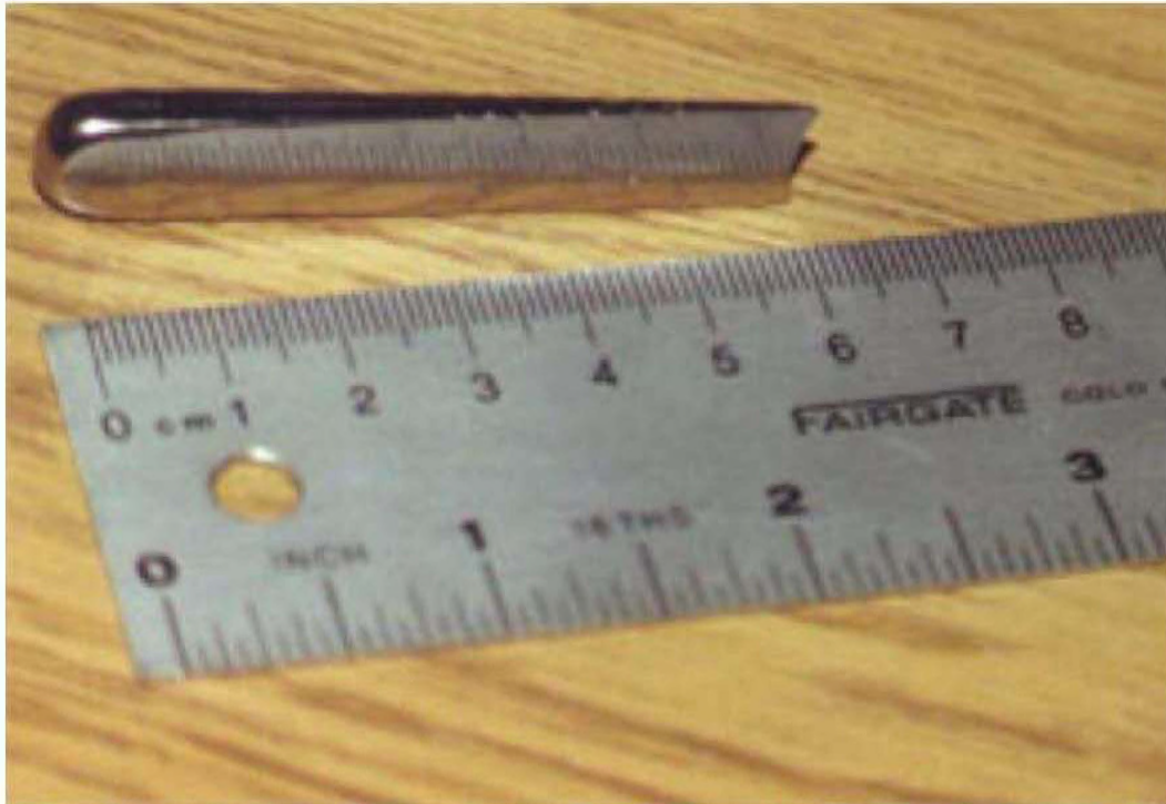
Figure 7. Cast Metallic Glass Wedge. Wedge of a zirconium-based bulk metallic glass produced by casting. Note the shiny metallic luster, typical of metallic glasses. 27
