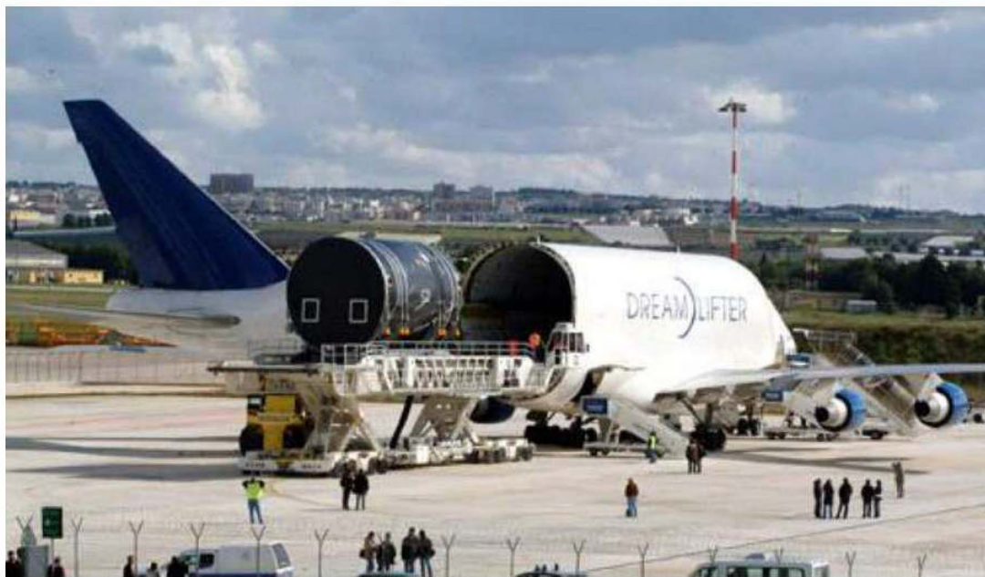
Figure 2. Specially Modified 747 Transporter Unloading a Boeing 787 Composite Fuselage Barrel Section
