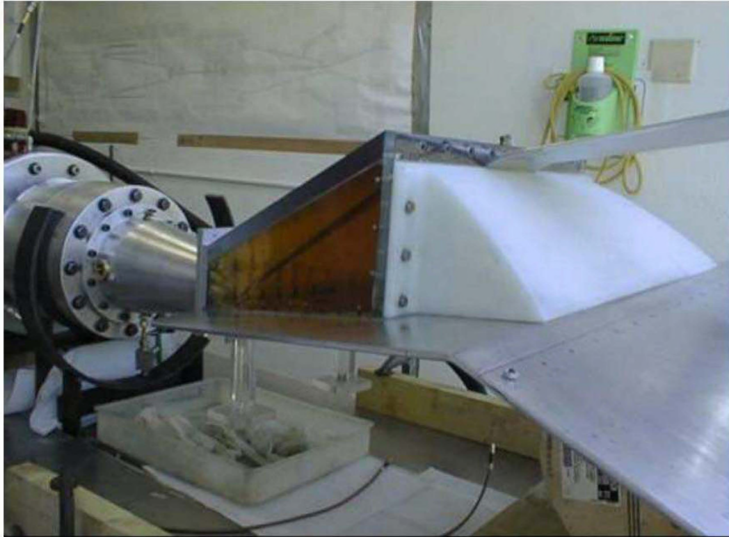
Figure 7. H5 Output Section With the Point Geometry Converter Feeding an Extended-Ground-Plane Antenna Through a Brewster Angle Window
