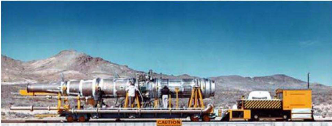
Figure 2. Tory-IIC Ready for Testing (courtesy LLNL)
