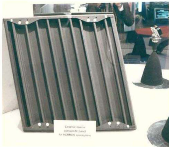
Figure 22. This 1988 SEP Bordeaux SiC/SiC Panel Could Sustain Temperatures of up to 3,000 °F. With SEP having subsequently closed, little of this capability remains.
