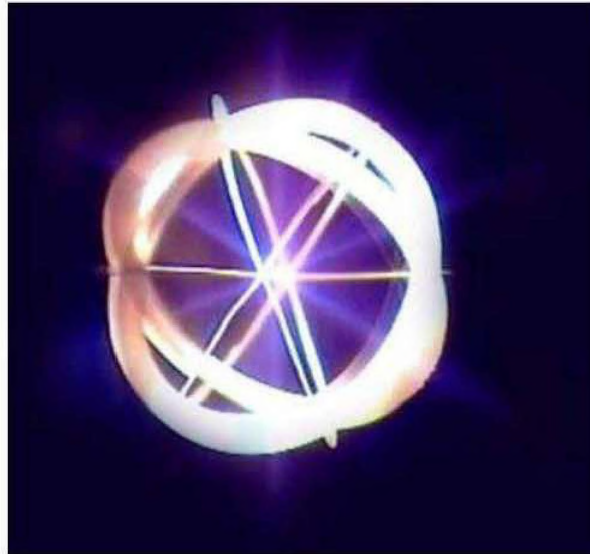
Figure 2.3. Photograph of a STAR mode discharge. The "vane" type grid shown is only one of a number of large opening grids designed and used for STAR mode operation of the neutron source type IEC. This particular design (but with variations) has been used by the UIUC, Daimler-Chrysler and Kyoto University. It is rugged, shows little sputtering and has proven very efficient for neutron production. Materials used vary from stainless steel to Mo.
