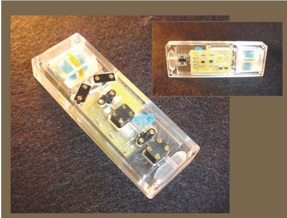
Figure 33. NASA Space Application of Microfluidic Cell Culture System Made by Micromachining (Towe - ASU research)
