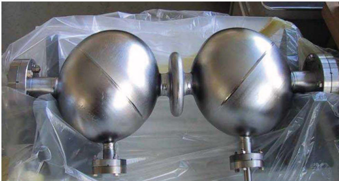
Figure 10. INFN Genoa HFGW Detector
