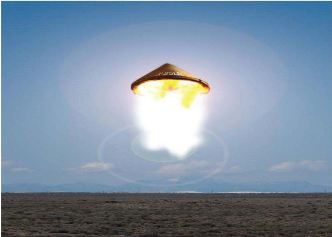
Figure 1. Air Force X-25LR Laser Lightcraft (courtesy of F. Mead, AFRL/PRSP, Edwards AFB, CA).
