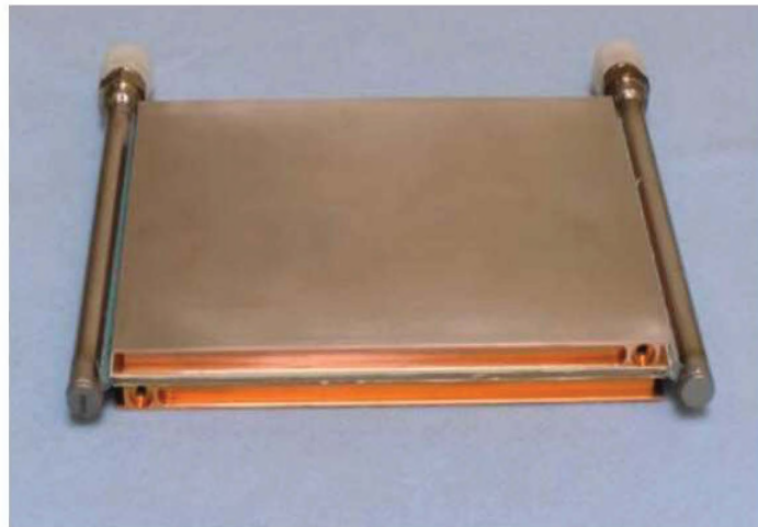
Figure 21. Phase Change Materials Allow Storage of Large Intermittent Heat Loads While Slow Regeneration Removes Heat from Aircraft (courtesy of P. Saunders, AFRL/RDS, Kirtland AFB, NM).
