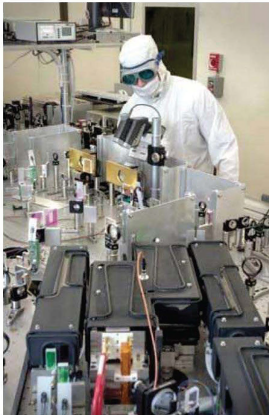
Figure 19. Northrop Grumman's Joint High Power Bulk Slab Solid-State Laser (courtesy of the Directed Energy Professional Society).
