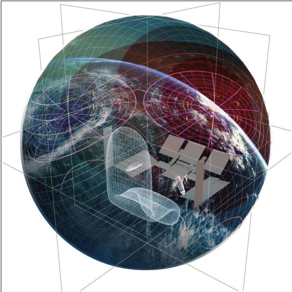
Figure 13. Provisional Breakthrough-Era Cockpit. The spherical zone around the cockpit center represents the virtual surround display onto which images of the environment outside the vehicle are displayed. Keeping with lessons of prior human interfaces, a minimal set of physical displays are also provided, with the most important ones located deliberately in the “tunnel vision” zone in front of the pilot. [Graphic: A. Szames with background image through M. Cherfi]
