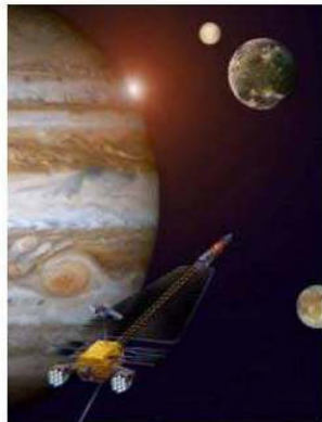
Figure 13. Nuclear Electric Propulsion (NEP) Concept Vehicles. Left is the 100-kWe Jupiter Icy Moons (JIMO) planetary spacecraft. Right is a 100-MWe-class piloted Mars vehicle.
