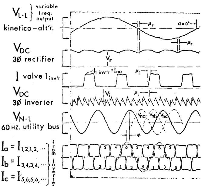
Fig. 4. Waveforms of voltages and currents along the asynchronous link. Case III: Kinetic-alternator speed  $\approx 0.28$  pu.  $V, I, P, \approx 1.0$  pu.
