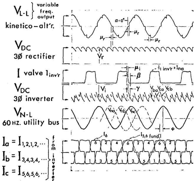
Fig. 2. Waveforms of voltages and currents along the asynchronous link. Case I: Kinetic-alternator speed  $\approx 1.0$  pu.  $V, I, P, \approx 1.0$  pu.
