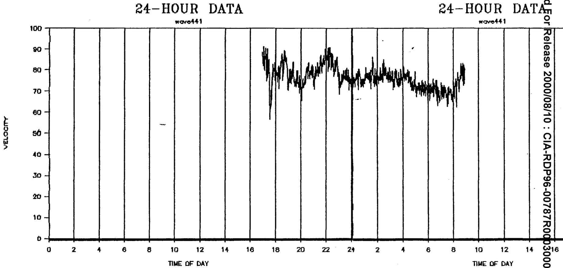
Fig. 4 Overnight data from the flow system after upgrading to 12 bit data transfer
