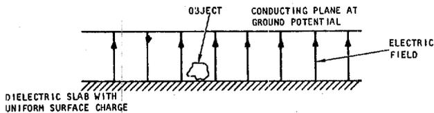
Figure 1. Electric Field Between Parallel Plates
