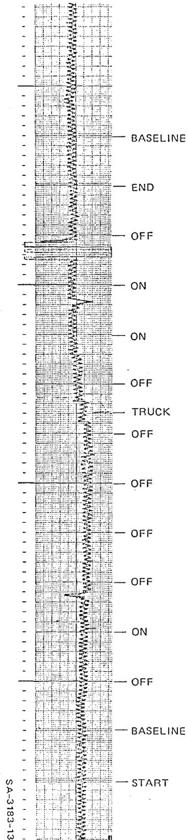
discussed below. An artifact due to the passage of a truck in the parking lot adjacent to the laboratory (under continuous surveillance by the experimenter) is noted in period 6. Each of the signals on scale corresponds to an input  $\sim 1.6 \times 10^{-9}$  Gauss/cm<sup>2</sup> (second derivative  $\partial^2 B_z / \partial z^2$ ), which is equivalent to  $\sim 3.5 \times 10^{-7}$  Gauss referred to one pickup coil.
