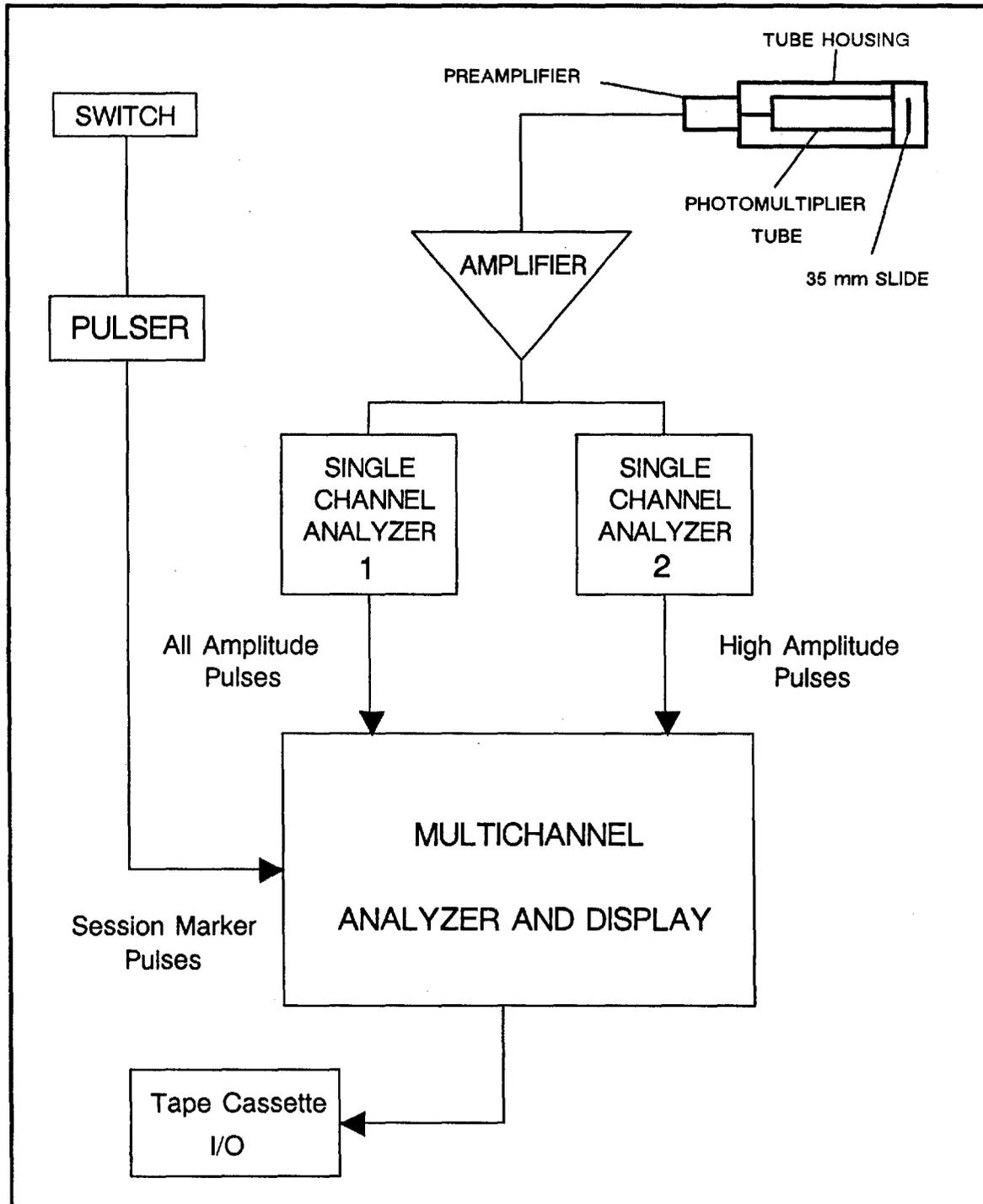
Figure 1 SCHEMATIC DIAGRAM FOR THE PHOTON PRODUCTION EXPERIMENT
