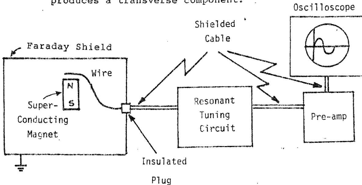
Figure 7. A sensitive scalar wave detector.
