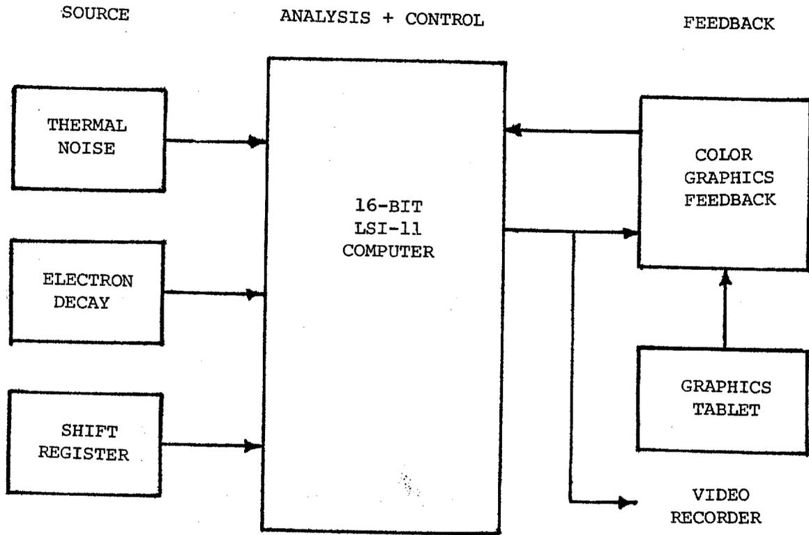
FIGURE 1: BLOCK DIAGRAM OF A COMPUTER-BASED INSTRUMENT DESIGNED TO BE SENSITIVE TO REMOTE PERTURBATION PROCESSES
