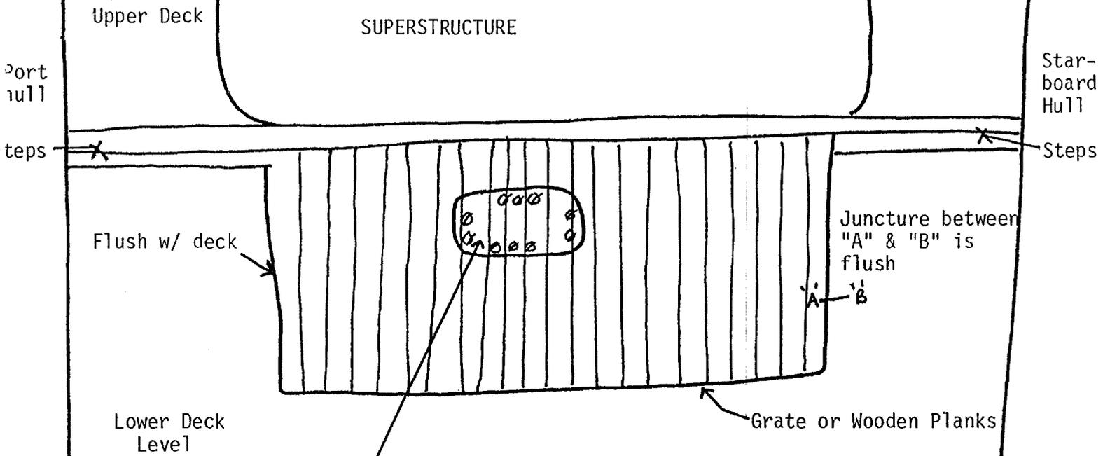
\*Opening to hidden compartment; securely bolted/screwed down with water tight seal. Compartment inside has a false bottom made to look like a storage bin/hold/bay. Beneath this false bottom is an extensive sub-level(s) which has been densely packed with the blue-wrapped packages described in text.
