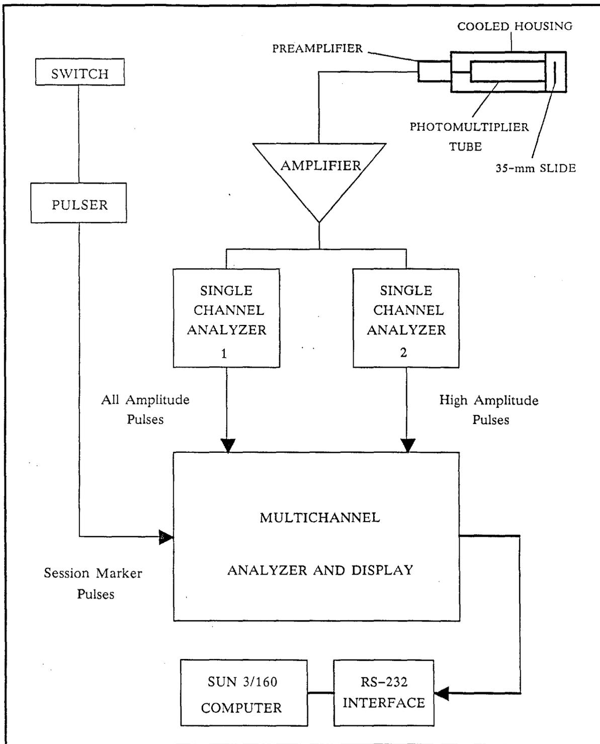
FIGURE 1 SCHEMATIC DIAGRAM FOR PHOTON PRODUCTION EXPERIMENT
