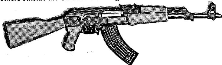
■ **THE AK-47** is a compact weapon of Soviet origin. It is supplied in two versions, one with a rigid butt and one with a double-strut folding metal butt-stock. The military version is fully automatic.
