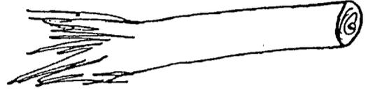
Broken wood; end appears like a tree trunk which has exploded at one end.
