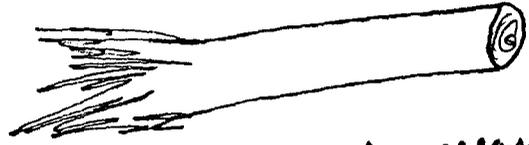
Broken wood; end appears like a tree trunk which has exploded at one end.
