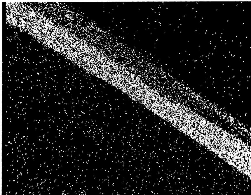
Figure 31. SEM-X Zinc X-ray Map of Warm-Formed Cross-Section
